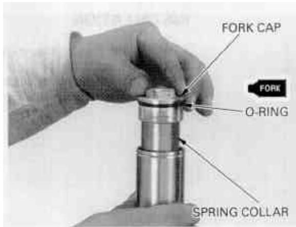
Hold the fork cap and tighten the lock nut to the specified torque.
