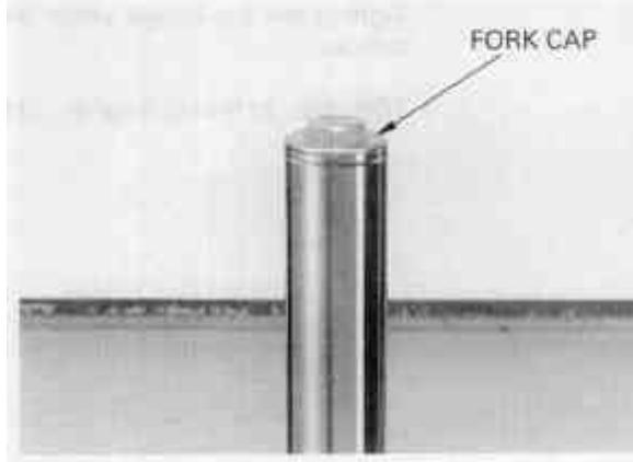
Install the fork protector onto the fork slider aligning the protector boss with the groove in the fork slider.
