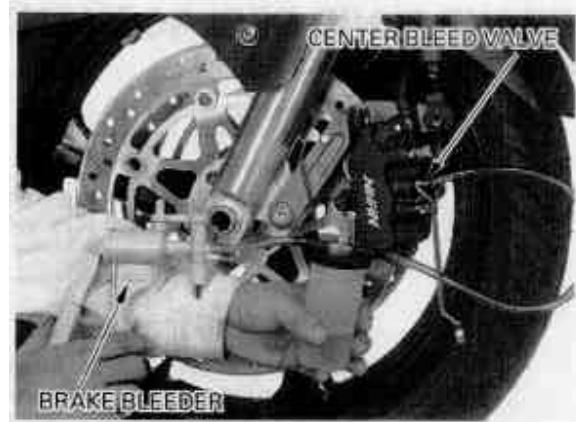
Connect a commercially available brake bleeder to the rear brake caliper outer bleed valve.
