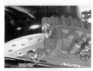
Install and tighten the pad pin plug.
