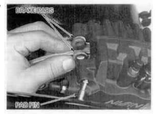
Tighten the pad pin to the specified torque.
