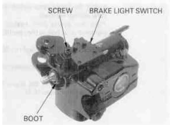
Apply silicone grease to the contact surface of the master piston, then install the brake lever assembly.
