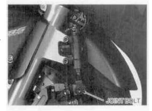
Remove the brake hose oil bolt, sealing washers, brake hose eyelet.
