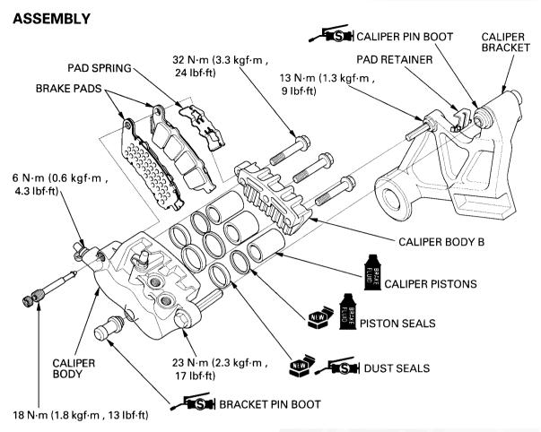
Coat the new piston seals with clean brake fluid. Coat the new dust seals with silicone grease.
