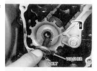
Shift the transmission into 6th gear and apply rear brake.
