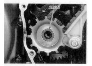
Apply oil to the ignition pulse generator rotor bolt threads, then install the washer and rotor bolt.
