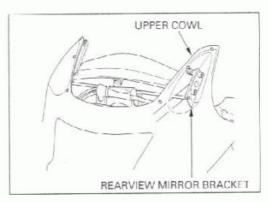
Disconnect the headlight sockets, then remove the upper cowl.
