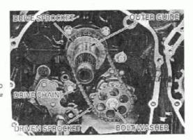
Remove the three flange bolts and oil pump assembly.
