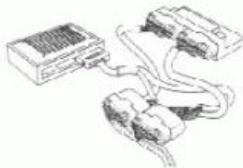
Crank the engine with the starter motor, and measure the ignition pulse generator peak voltage at the test pin box terminals.
