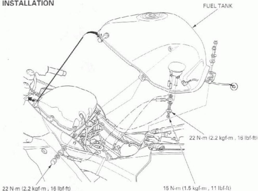
Connect the fuel hose to the fuel pump with new sealing washers.
