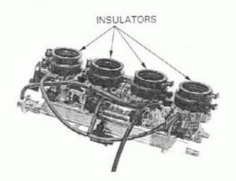
Apply oil to the insulator inside surfaces for ease of throttle body installation.
