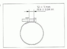
Connect the water hoses to the fast idle wax unit, tighten the clamp scrow securely.
