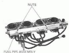
Remove the injectors from the throttle body.
