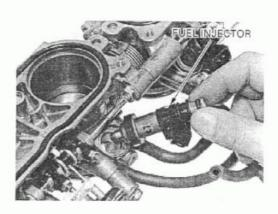
Remove the seal ring, O-ring and cushion ring.
