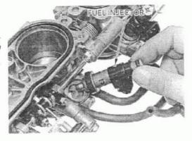
Install the fuel pipe assembly over the fuel injectors.
