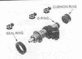
Install the fuel injectors into the throttle body.
