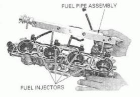
Install and tighten the fuel pipe mounting nut to the specified torque.
