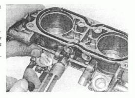
Remove the wax unit link bracket screw.
