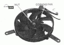
Install the fan motor/cooling fan assembly onto the radiator.
