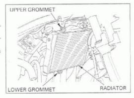
Install and tighten the radiator mounting bolt.
