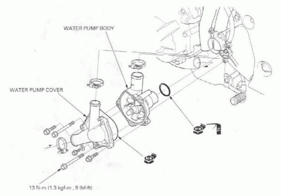
Connect the water pump-to-water joint hose to the water pump and tighten the clamp screw.
