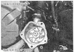
Apply engine oil to a new O-ring and install it onto the stepped portion of the water pump.
