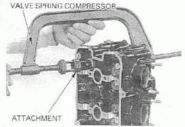
Tap the valve stems gently with two plastic hammers as shown to seat the cotters firmly.
