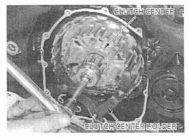
Remove the lock washer, thrust washer and clutch center.
