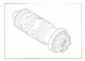
Turn the inner race of the shift drum bearing with your finger.
