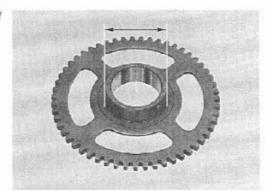
Check the one-way clutch for wear or damage and replace if necessary.
