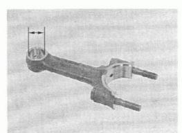
Temporarily install the connecting rod to the crankshaft.
