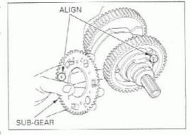
Apply molybdenum disulfide oil to the area shown in the illustration.
