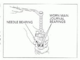
Press a new needle bearing onto the crankshaft using a hydraulic press and special tool.
