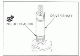
If the special tool is not available, prepare a suitable collar, washer and 8 mm flange bolt (example; flywheel bolt) for the bearing installation. Assemble the above items, and screw the bolt gradually, then install the new needle bearing.
