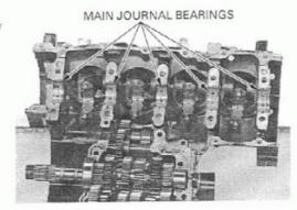
Wipe the oil from the bearing inserts and journals. Reinstall the upper crankcase's main journal bearing inserts, then carefully lower the crankshaft in place.
