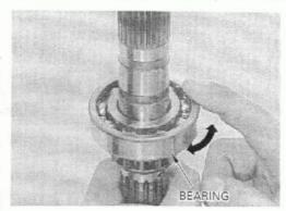
Press out the mainshaft from the bearing using a hydraulic press.
