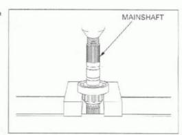
Install a new mainshaft bearing onto the mainshaft by pressing the mainshaft bearing inner race using the special tool.
