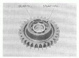
Press the new idle gear bearing into the idle gear using the special tools.
