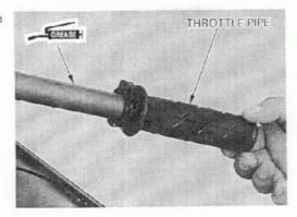
Apply grease to the throttle cable ends and sliding surface.
