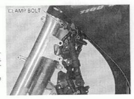
It is not necessary to remove the oil bolts and oil pipe from the dalay valve. For the right fork leg removal, remove the brake pipe 3 way joint mounting bolt, then the delay valve mounting bolts and reflector.
