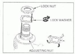
Install and finger tighten the lock nut.
