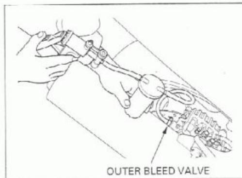
Connect a commercially available brake bleeder to the rear brake caliper center bleed valve.
