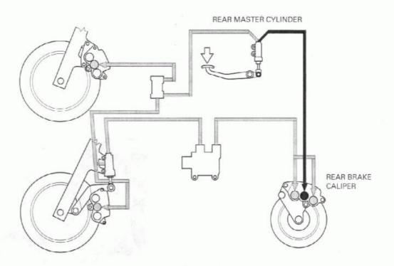
Feed the brake fluid at the rear brake caliper center bleeder valve as same procedure in step 1.
