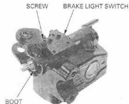
Apply silicone grease to the contact surface of the master piston, then install the brake lever assembly.
