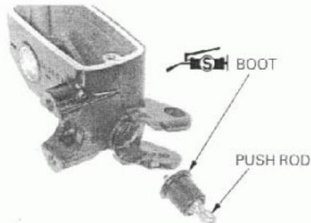
Install the brake light switch and tighten the screw to the specified torque.
