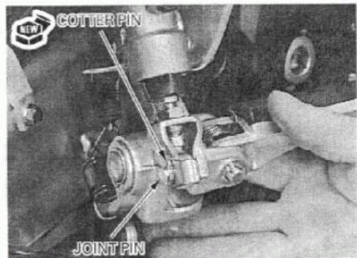
Install the right footpeg assembly onto the frame.
