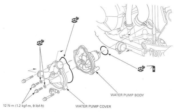
Apply engine oil to a new O-ring and install it onto the stepped portion of the water pump body.
