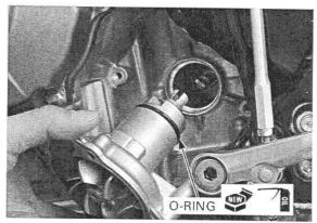
Install the water pump body into the crankcase while aligning the water pump shaft groove with the oil pump shaft end by turning the water pump impeller.
