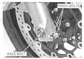
Install the both brake caliper and tighten the new mounting bolts to the specified torque.
