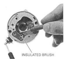
Check for continuity between the cable terminal and the rear cover.
