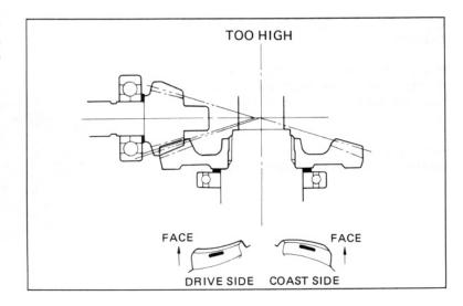
Replace the pinion spacer with a thinner one if the contacts are too low, to the flank side. The patterns will shift about 1.5–2.0 mm (0.06–0.08 in) when the thickness of the spacer is changed by 0.10 mm (0.004 in).
