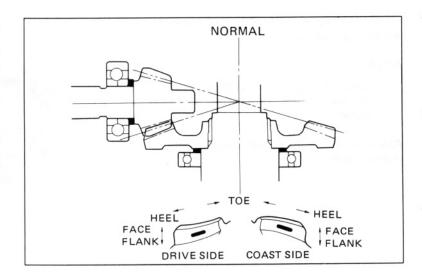
If the patterns are not correct, remove and replace the pinion spacer. Replace the pinion spacer with a thicker one if the contacts are too high, toward the face.
