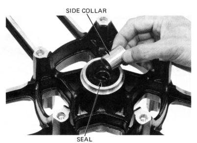
Remove the left seal and speedometer gear retainer.
