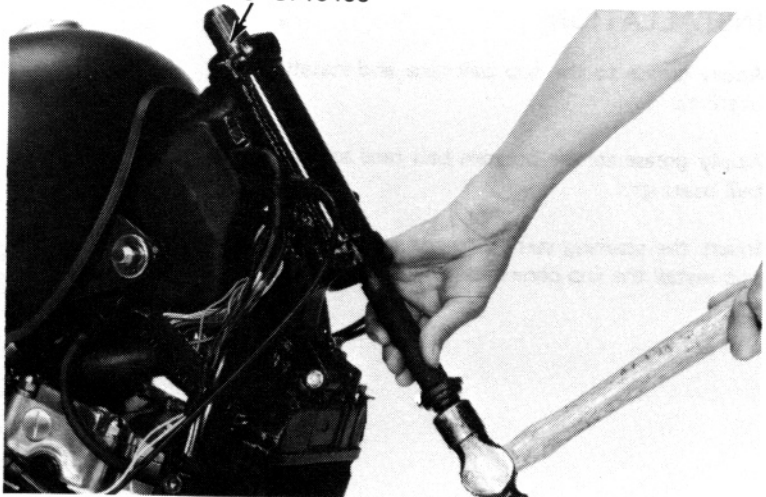
BEARING RACE REMOVER/ INSTALLER 07946-3710400
