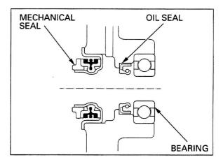
Remove the oil seal and mechanical seal from the right crankcase cover.
