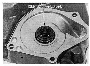
Drive a new mechanical seal using the special tool.
