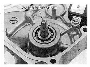
Remove the bearing using the special tools.
