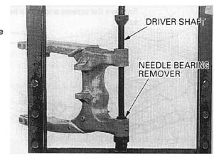
Press in the bearing with the marking side facing up.
