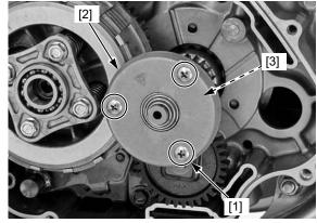
Remove the clip [1] while holding the oil through [2]. Remove the oil through and spring [3].
