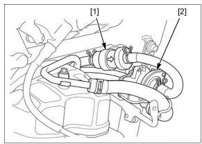
Check the PAIR hoses [1] between the air cleaner sub filter and air inlet cover for deterioration, damage or loose connections.
