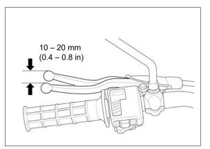
Minor adjustment are made with the upper adjuster at the clutch lever.
