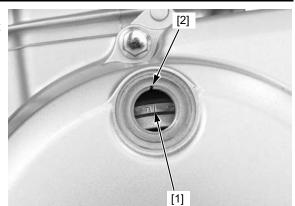
Coat a new O-ring [1] with engine oil and install it onto the timing hole cap [2].
