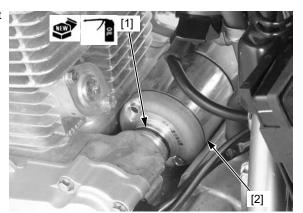
Install the mounting bolts [1] with the battery (–) cable [2] as shown, and tighten the bolts.
