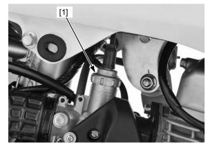
Be careful not to damage the jet needle [1] when removing the throttle valve [2] from the carburetor body.
