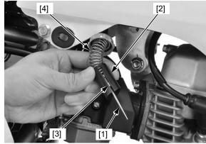
Turn the jet needle retainer [1] counterclockwise.
