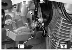
Loosen the connecting boot band screw [1]. Remove the carburetor mounting nuts [2] and wire clamp [3], then remove the carburetor [4] from the insulator.
