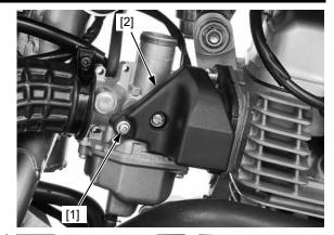
Except CO, III LA Disconnect the carburetor heater connector [1] and types: ground wire connector [2].
