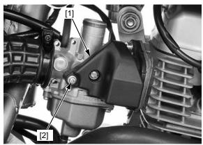
Connect the fuel hose [1] to the fuel valve. After installing the carburetor, check the following:
